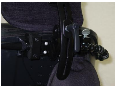
Flex Arm Holder for Slide-Track Mounted on rails on the Back of the Wheelchair
