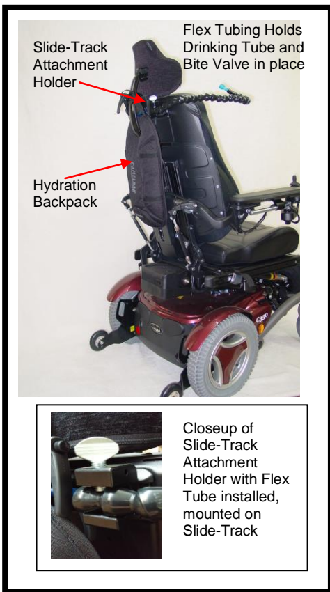
Hydration Backpack with Tube Positioning Mounted on a Powered Wheelchair
