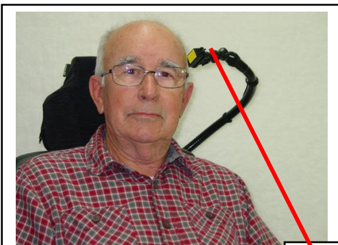
The Micro Light Adaptive Switch Mounted on a 6-inch Flex Arm Mounting System Using a Micro Light Adaptive Switch Mounting Kit to Position the Switch for Head Access for a Wheelchair User. Insert shows the parts provided in the Kit
