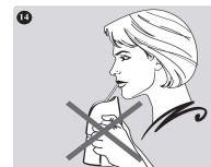
Fig. 14 Drinking from RiJe Cup through a straw in the cup's upright position will result in limited flow delivery instead of fixed dosage delivery.
